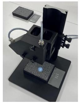
Now once again, the message with the prompt for the measurement period appears, i.e. over what period of time measurement values of the recyclate surface are to be averaged. In our example, this would once again be 30 s. Confirm with **OK**. Here too, the following applies: during the 30 s, the recyclate must be moved in the x- and y-direction (in inline operation, the vibrating chute takes care of the movement of the
