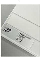
and place it with its rear side up on the upended recyclate holding bowl, or inline in the sliding carriage provided for the purpose, and once this has been done, acknowledge with **OK**. Please note: The distance between the sensor front end and RAL 9003-P should be 75 mm.
